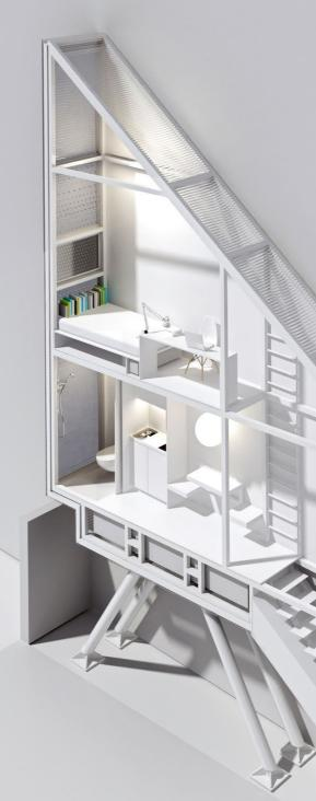
Top left Keret House provides enough space for an artist to sleep, eat, and work. Bottom left A narrow desk provides a mini-workspace. Bottom middle The translucent facade is visible above an existing wall. This page The triangular-shaped structure is elevated off the ground and slots between two existing residential buildings.
