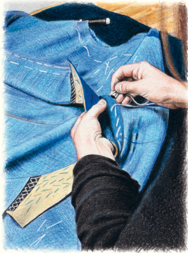
Basting a collar onto a fitting.
