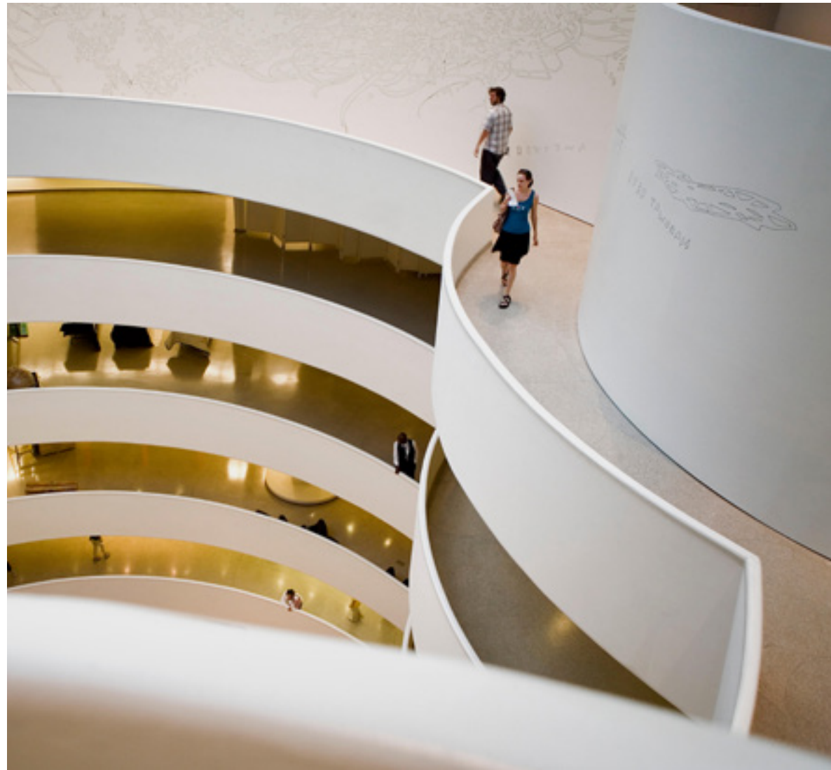
A quarter-mile of cantilevered concrete ramps climb the museum's outer walls. The building's domed skylight, or "oculus," consists of twelve sections resting on concrete structural columns that extend down through the building.
